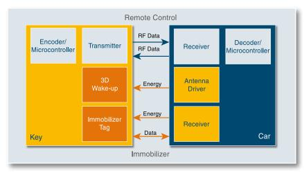
Bi-directional RF link for the RKE function as well as for the extremely secure duplex RF link in a Passive Entry Go system. The IF link is used for the wakeup channel in a PEG system as well as for the immobilizer function to start the RF communication.
