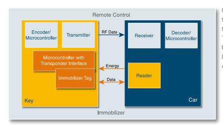
Uni-directional RF link for the keyless entry function to open or lock the doors. The immobilizer system is built with a bi-directional LF link operating with the AUT64 crypto algorithm.
