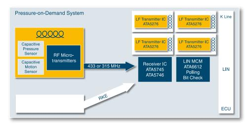
A POD system is a master/slave system. In addition to direct TPMS systems, it includes a 125-kHz built-in channel for waking up sensor modules in defined duty cycles. Such systems remarkably increase the
