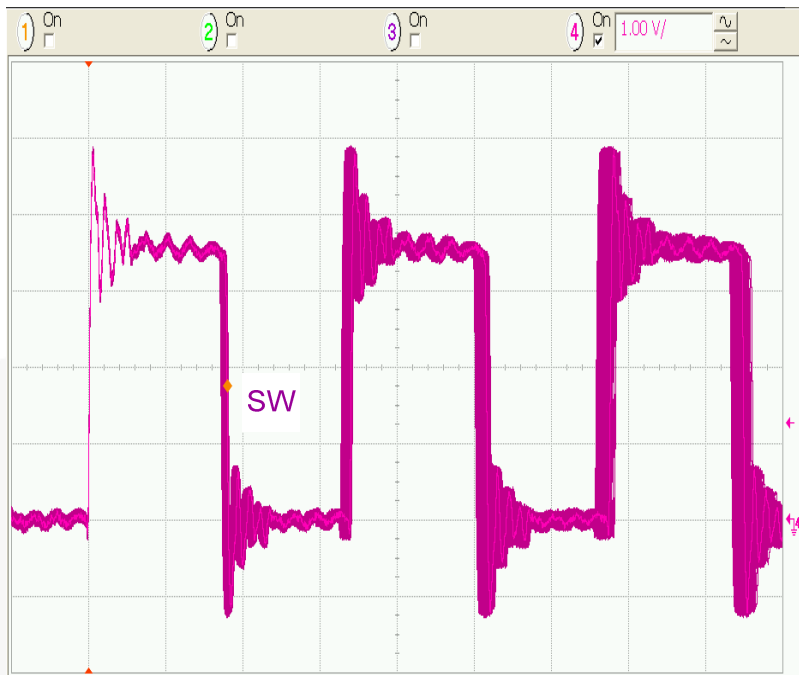
Figure 38. SW-Node Jitter (Infinite Persistence), I_{LOAD} = 200mA , 50ns/div.
