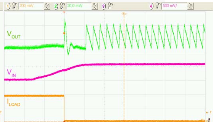
Figure 22. Combined Line/Load Transient 3.3 to 3.9V_{IN} Combined with 400mA to 40mA Load Transient
