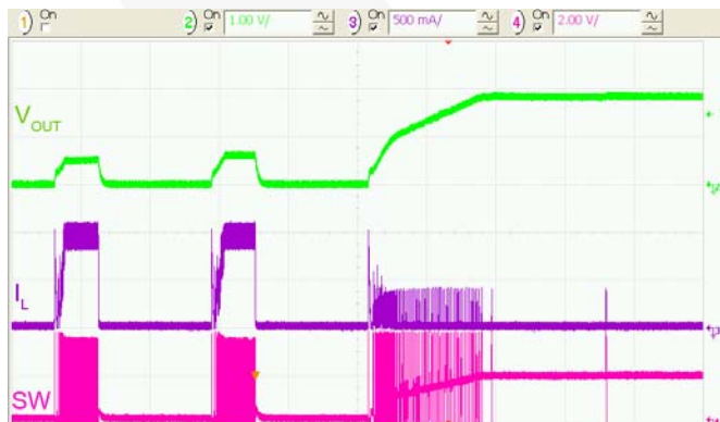
Figure 36. Overload Recovery to Light Load, 50\mu s/div.
