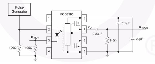
Figure 15. Test Schematic
