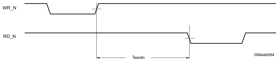
Fig 17. ISP1582 ready signal timing
