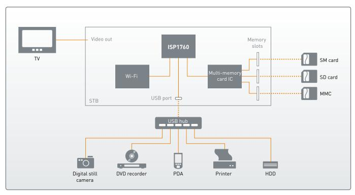
Embedded in a set-top box, the ISP1760 creates a hub for conveniently viewing high-resolution pictures or video clips, and then saving and printing them.
