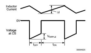
FIGURE 3. CS Pin Waveform
