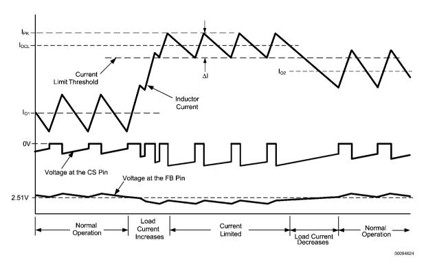
FIGURE 2. Normal and Current Limit Operation
