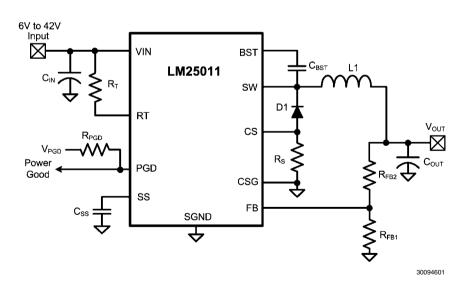
M25011 42V, 2A Constant On-Time Switching Regulator with Adjustable Current Limit
