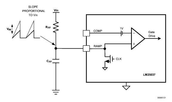
FIGURE 4. Feed-Forward Voltage Mode Configuration
