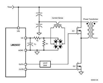
**FIGURE 12. Current Sense Using Transformer**
