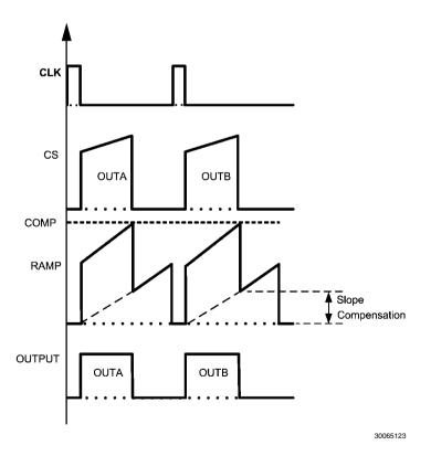
FIGURE 6. Timing Diagram for Current Mode Configuration
