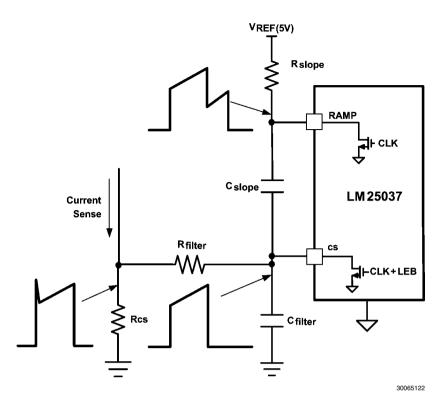
FIGURE 5. Current Mode Configuration with Slope Compensation
