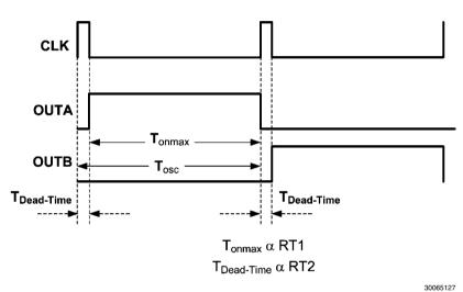
FIGURE 7. Timing Diagram of OUTA, OUTB and Dead-Time Set by RT2
