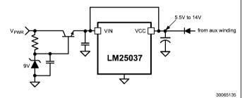
FIGURE 11. Start-up Regulator for VPWR >75V
