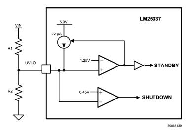
FIGURE 14. Basic UVLO Configuration
