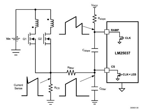
**FIGURE 9. Current Mode Configuration**
