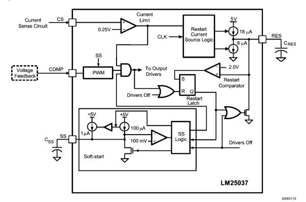
FIGURE 2. Current Limit Restart Circuit
