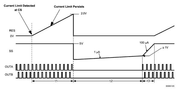
FIGURE 3. Current Limit Restart Timing
