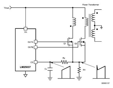
FIGURE 13. Current Sense Using Current Sense Resistor (R1)
