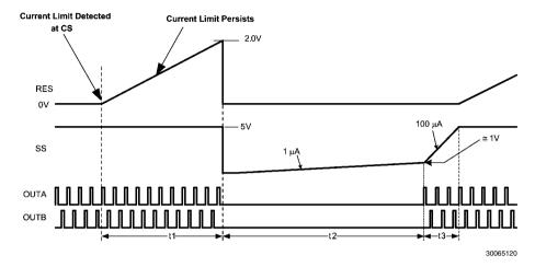
FIGURE 16. Hiccup Over-Load Restart Timing
