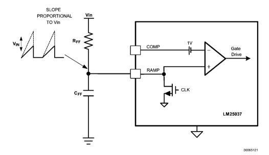
FIGURE 8. Feed-Forward Voltage Mode Configuration
