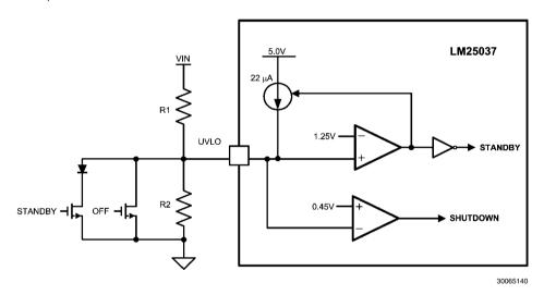
FIGURE 15. Remote Standby and Disable Control
