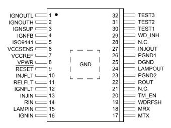
Figure 4. 33812 Pin Connections
