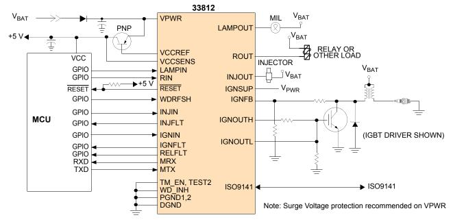
Figure 1. 33812 Simplified Application Diagram
