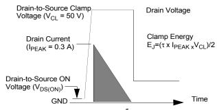
Figure 5. Output Voltage Clamping
