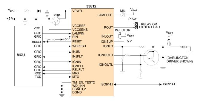
Figure 2. 33812 Simplified Application Diagram (Darlington Mode)
