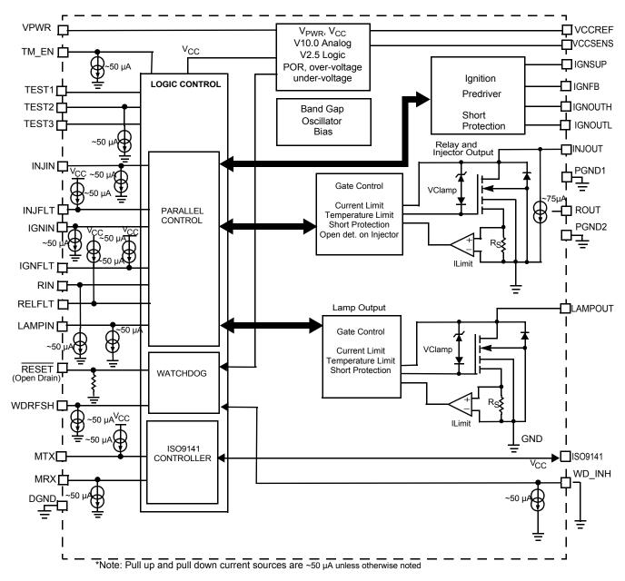
Figure 3. 33812 Simplified Internal Block Diagram
