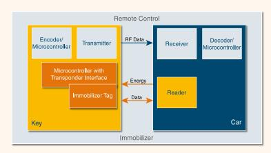
Uni-directional RF link for the keyless entry function to open or lock car doors. The immobilizer system is built with a bi-directional LF link operating with the AUT64 crypto algorithm.
