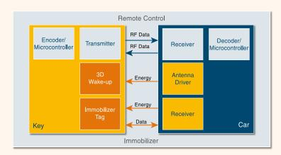
Bi-directional RF link for RKE functions as well as for the extremely secure duplex RF link in a Passive Entry Go (PEG) system. The IF link is used for the wake-up channel in a PEG system as well as for the immobilizer function to start the RF communication.
