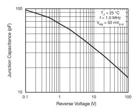
Fig. 5 - Typical Junction Capacitance
