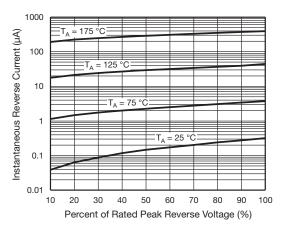
Fig. 4 - Typical Reverse Leakage Characteristics
