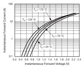
Fig. 3 - Typical Instantaneous Forward Characteristics
