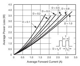
Fig. 2 - Average Power Loss Characteristics
