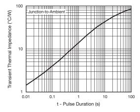
Fig. 6 - Typical Transient Thermal Impedance
