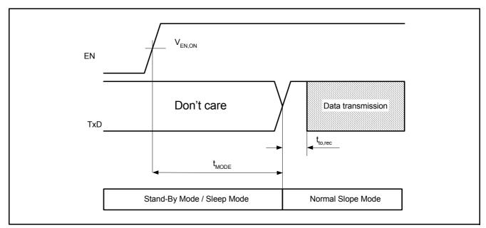
Figure 5 Timing to enter Normal Slope Mode
