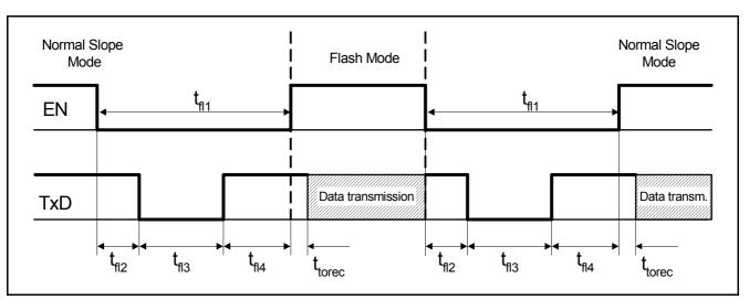
Figure 6 Timing to enter and leave Flash Mode
