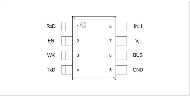
Figure 2 Pin Configuration IFX1021SJ
