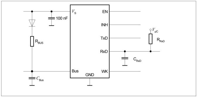
Figure 12 Simplified test circuit for static characteristics
