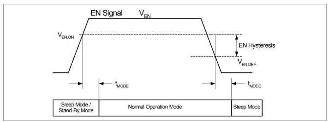
Figure 9 Mode Transition via EN pin
