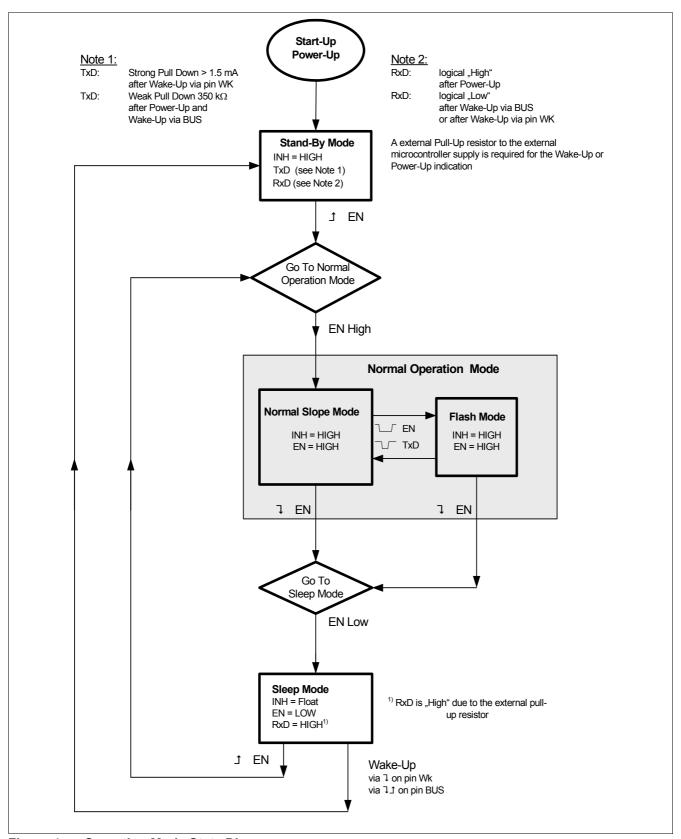
Figure 4 Operation Mode State Diagram
