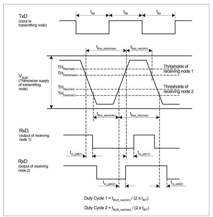
Figure 13 Timing diagram for dynamic characteristics
