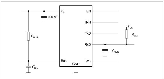
Figure 11 Simplified test circuit for dynamic characteristics
