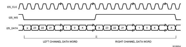
FIGURE 7. I2S Normal Input Format
