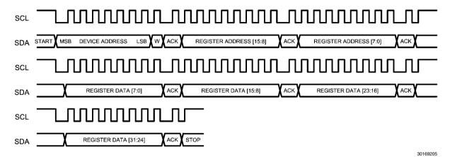
FIGURE 5. Example I<sup>2</sup>C Write Sequence
