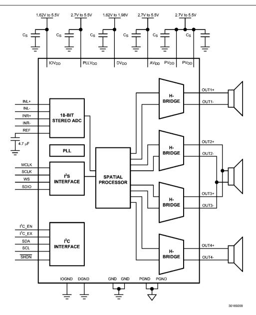
FIGURE 2. Channel Audio Amplifier Application Circuit
