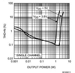
THD+N vs OUTPUT POWER  $\label{eq:RL} \textbf{R}_{L} = 4\Omega, \, f = 1 \text{kHz}, \, \text{ADC Input, All channels}$
