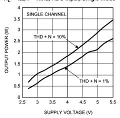
OUTPUT POWER vs SUPPLY VOLTAGE  $R_L = 8\Omega$ , f = 1kHz, ADC Input, Single channel
