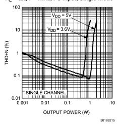
THD+N vs OUTPUT POWER  $R_L = 8\Omega$ , f = 1kHz, ADC Input
