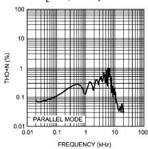
THD+N vs FREQUENCY  $V_{DD} = 3.6V, P_{OUT} = 450mW,$  $R_L = 8\Omega$ , I<sup>2</sup>S Input
