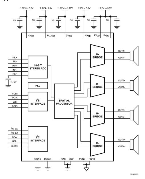
FIGURE 1. Typical Audio Amplifier Application Circuit
