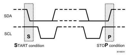
FIGURE 4. Start and Stop Diagram
