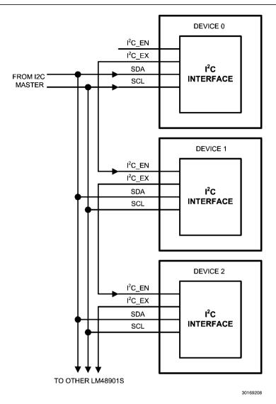
FIGURE 11. I<sup>2</sup>C\_EN/I<sup>2</sup>C\_EX Daisy Chaining Example
