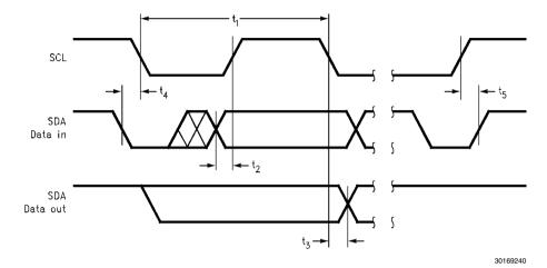
FIGURE 3. I2C Timing Diagram
