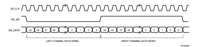
FIGURE 8. I2S Left Justified Input Format
