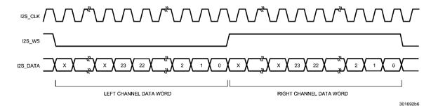
FIGURE 9. I2S Right Justified Input Format
