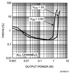
THD+N vs OUTPUT POWER  $R_L = 8\Omega, \, f = 1 \text{kHz}, \, l^2 S \, \text{Input, Single mode}$
