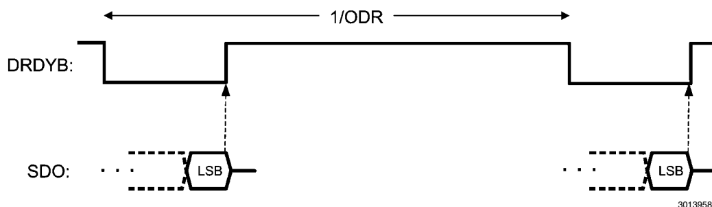
FIGURE 20. DRDYB Behavior for a Complete ADC_DOUT Reading
