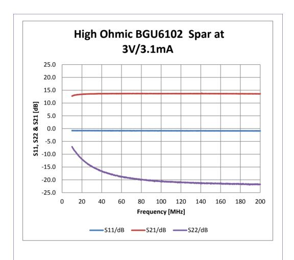
Fig 4. Gain, Input and Output Matching
