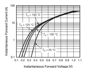
Fig. 2 - Typical Instantaneous Forward Characteristics
