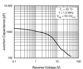
Fig. 4 - Typical Junction Capacitance
