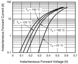
Fig. 2 - Typical Instantaneous Forward Characteristics
