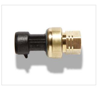
bonding process. Regarding their assembly sensors with different pressure ranges distinguish themselves only through membranes with different thickness as well as electronic calibration. On both ceramic parts there is a thin gold layer that is connected to the electronics via contact leads. Both gold layers form a capacitor with its capacity changing as a function of pressure put onto the membrane. The capacitor's capacity is in the 15 pF range.
