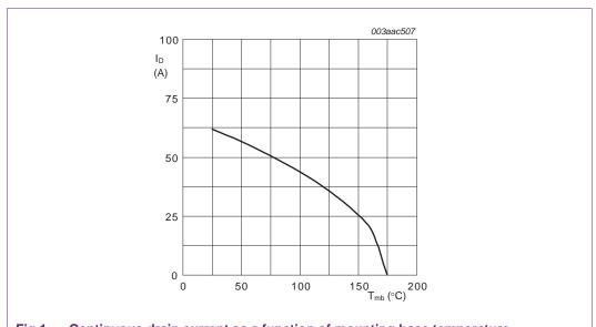
Fig 1. Continuous drain current as a function of mounting base temperature
