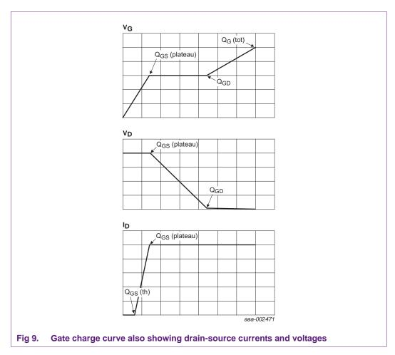
Because the capacitance varies with voltage and current, it is better to look at the gate charge data than the capacitance data when determining switching performance. This is especially true if the gate-driver circuit for the MOSFET is limited to a particular current, and a rapid switch is required.
