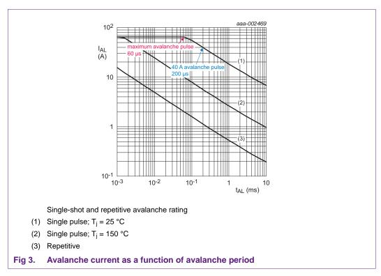
A simple example for the BUK7Y12-55B, using the information in *AN10273*, is extracted from the limiting values Table 3:
