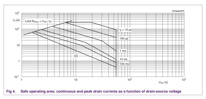
The SOA curves show the voltage allowed, the current and time envelope of operation for the MOSFET. These values are for an initial  $T_{mb}$  of 25 °C and a single current pulse. This is a complex subject which is further discussed in the appendix (Section 3.1).
