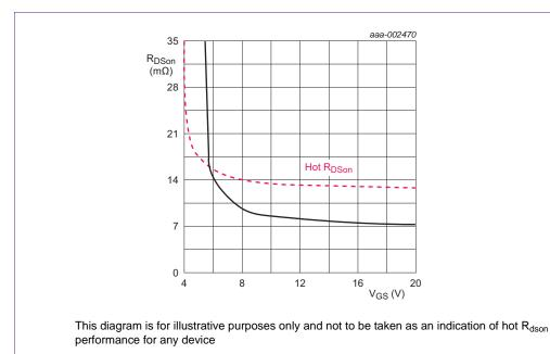
Fig 7. Drain-source on-state resistance as a function of gate-source voltage at 25 °C and high temperature
