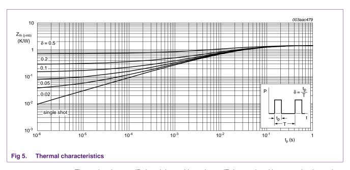
Thermal resistance ( $R_{th}$ ) and thermal impedance ( $Z_{th}$ ) are related because the thermal resistance is the steady-state measure of how the device blocks heat flow. Thermal impedance is how the device responds to transient thermal events. It involves different thermal capacities of parts of the device and the thermal resistances between these parts. Under DC conditions,  $Z_{th}$  is equal to  $R_{th}$ . Equation 4 represents the temperature rise for a particular power dissipation:
