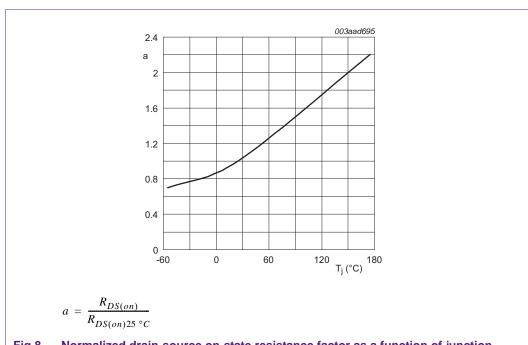
Fig 8. Normalized drain-source on-state resistance factor as a function of junction temperature
