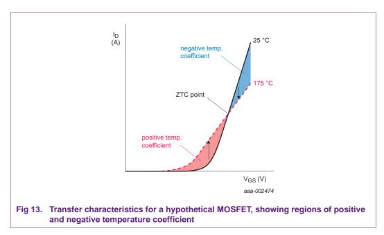
The resistance increase dominates at high currents, meaning that localized heating leads to lower currents. The threshold-voltage drop dominates at low currents, meaning that localized heating lowers the threshold voltage. This condition effectively turns on the device more, leading to higher currents and a risk of thermal runaway.
