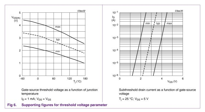
The first graph shows the variation in the threshold voltage for the typical and limit devices over the rated temperature range. All the MOSFETs are guaranteed to have a threshold voltage between the lines.
