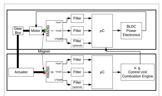
Fig. 12: System block diagram with two KMZ60 for BLDC motor and angular measurement application.
