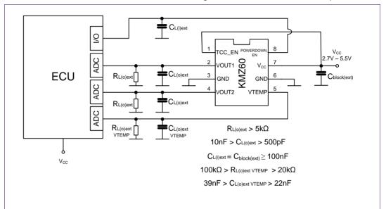
Fig. 17: Application circuit diagram for KMZ60 with Power-Down-Mode and TC compensation and temperature dependent output signal VTEMP.
