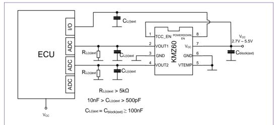
Fig. 16: Application circuit diagram for KMZ60 with Power-Down Mode and TC compensation.
