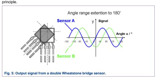
The two sensor bridges are positioned at an offset angle of 45° to each other. In this arrangement, two output signals show an electrical phase shift of 90°. The two signals are therefore proportional to  $\sin 2\alpha$  and  $\cos 2\alpha$ , respectively. It can be proved easily that these two signals now allow an evaluation of a 180° angular range.
