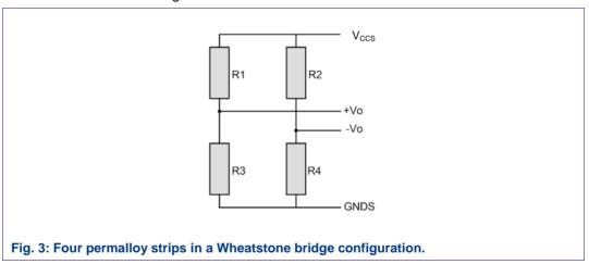
According to the basic relationship given by Equation (1), the differential output signal (+Vo, -Vo) of such a Wheatstone bridge is proportional to  $\sin 2\alpha$ . This means that a sensor comprising one Wheatstone bridge can measure an angular range of 90°. This is visualized in Fig. 4.
