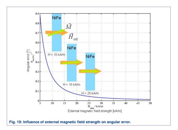
It is obvious that the measurement error caused by signal form errors can be neglected when using a magnetic field larger than 25kA/m.
