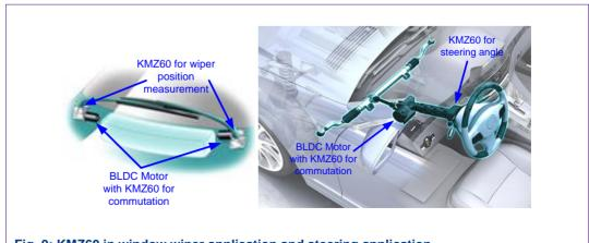
Fig. 9: KMZ60 in window wiper application and steering application.
