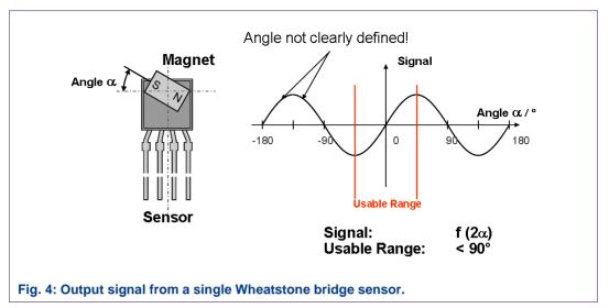
The limited angular range can be extended to 180° measurement range by using a two-bridge arrangement combined with a signal evaluation explained below. Fig. 5 shows the
