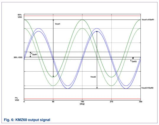
The output signal is valid between the output minimum limit of 7%  $V_{CC}$  and maximum limit of 93%  $V_{CC}$ .
