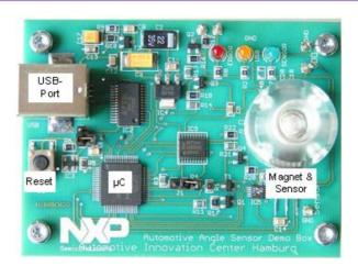
Fig. 23: KMZ60 hand-driven demo board.
