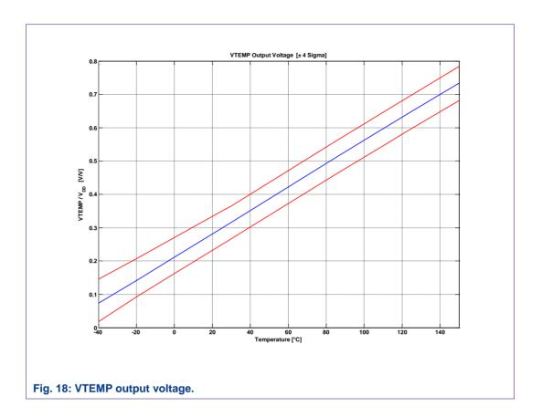
The internal temperature of the KMZ60 can be calculated from the output voltage in the following way:
