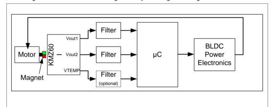
Fig. 11: System block diagram with KMZ60 for BLDC motor.
