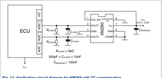
Fig. 14: Application circuit diagram for KMZ60 with TC compensation.
