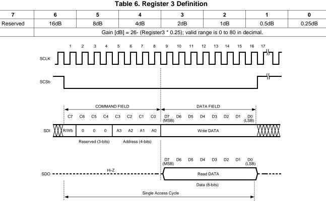
Figure 46. Serial Interface Protocol (SPI Compatible)
