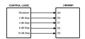
Figure 45. Parallel Mode Connection
