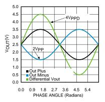
Figure 40. Differential Output Voltage
