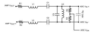
Figure 42. ADC Noise Filter Schematic
