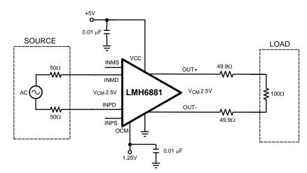
Figure 38. Typical Implementation with a Differential Input Signal
