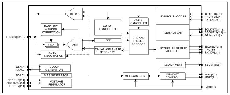
A member of Broadcom's third generation of Gigabit Ethernet PHYs, the **BCM5482** consists of two complete 10/100/1000BASE-T Gigabit Ethernet transceivers integrated on a single monolithic CMOS chip. The **BCM5482** is optimized for low power and small footprint size to reduce design complexity for space-constrained IP phone applications. For 10/100BASE-TX applications, the single package offers a compelling advantage over two single devices for Gigabit uplinks.
