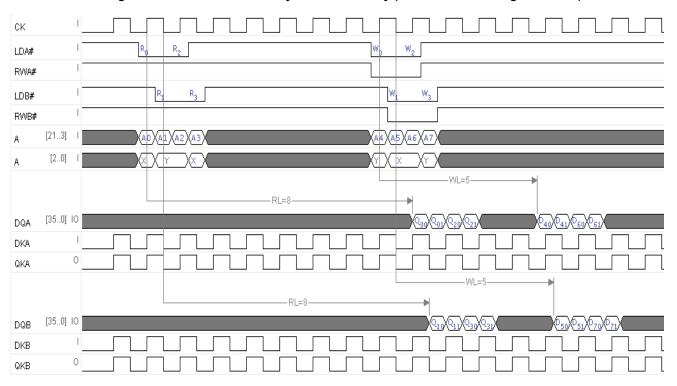
Figure 11. Waveforms for 8.0 Cycle Read Latency (Write to Read Timing Waveform)
