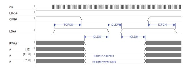
Figure 13. Configuration Read Timing Waveform
