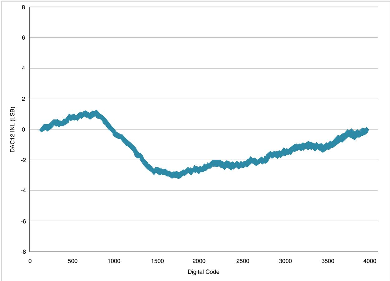
Figure 15. Typical INL error vs. digital code
