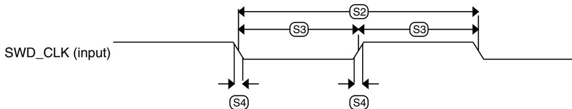
**Figure 4. Serial wire clock input timing**
