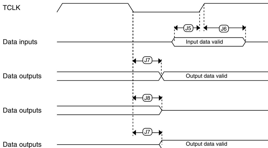
**Figure 7. Boundary scan (JTAG) timing**
