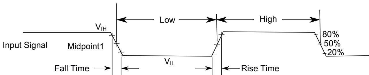
The midpoint is  $V_{IL} + (V_{IH} - V_{IL}) / 2$
