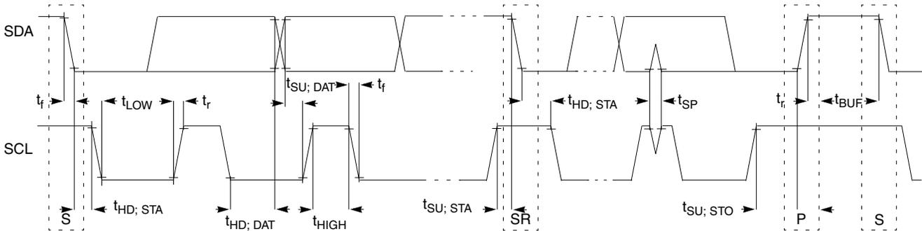
**Figure 21. Timing definition for fast and standard mode devices on the I<sup>2</sup>C bus**
