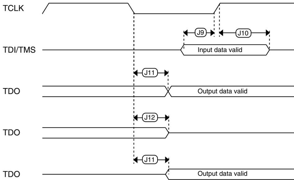
Figure 8. Test Access Port timing
