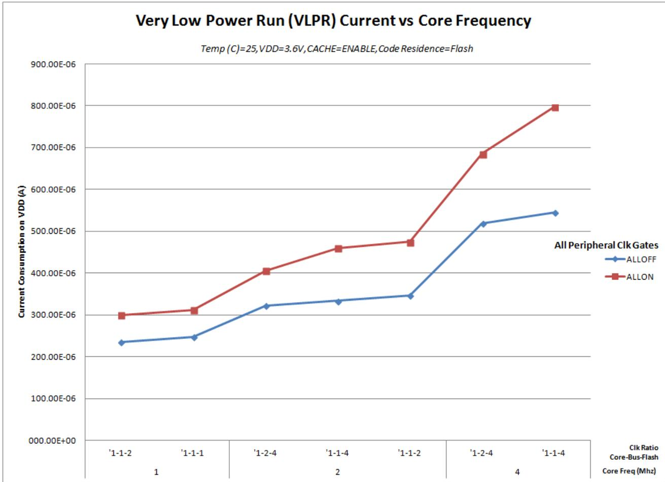
Figure 3. VLPR mode supply current vs. core frequency
