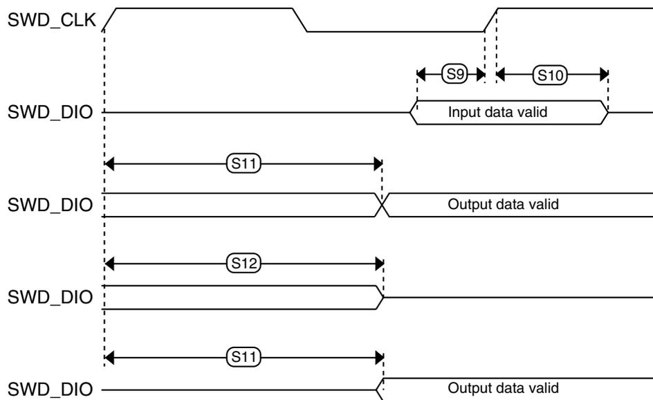
**Figure 5. Serial wire data timing**
