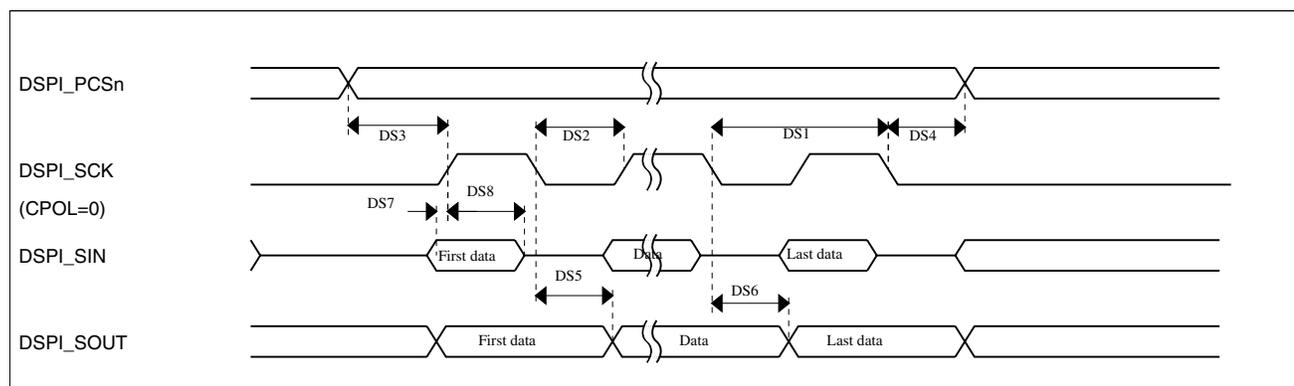
**Figure 17. DSPI classic SPI timing — master mode**
