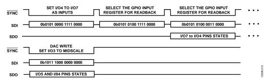
Figure 45. Configuring and Reading General-Purpose Input Pins
