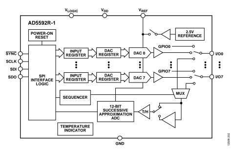
Figure 2. AD5592R-1 Functional Block Diagram
