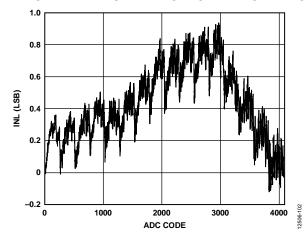
Figure 9. ADC INL,  $V_{DD} = 5.5 V$
