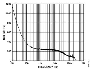
Figure 34. Reference Noise Spectral Density (NSD)
