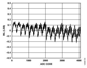
Figure 11. ADC INL,  $V_{DD} = 2.7 V$
