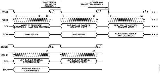
Figure 42. Multichannel ADC Conversion Sequence, No Repeat
