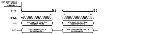
Figure 43. Multichannel, Repeating, ADC Conversion Sequence
