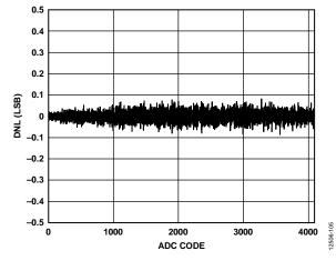
Figure 12. ADC DNL,  $V_{DD} = 2.7 V$
