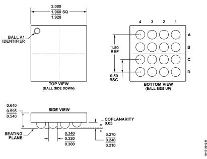
Figure 50. 16-Ball Wafer Level Chip Scale Package [WLCSP] (CB-16-3) Dimensions shown in millimeters
