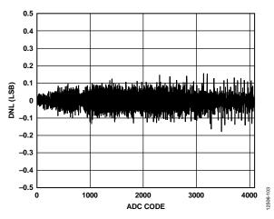
Figure 10. ADC DNL,  $V_{DD} = 5.5 V$
