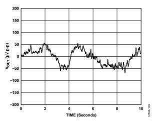
Figure 28. DAC 1/f Noise with External Reference
