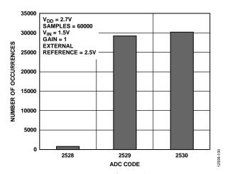
Figure 13. Histogram of ADC Codes,  $V_{DD} = 2.7 \text{ V}$
