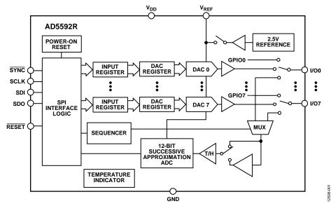
Figure 1. AD5592R Functional Block Diagram
