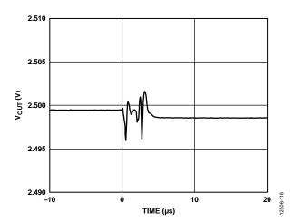
Figure 20. DAC Digital-to-Analog Glitch (Falling)
