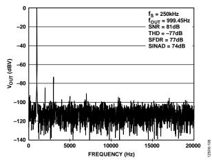
Figure 26. DAC Sine Wave Output, Output Range = 0 V to  $2 \times V_{REF}$ ,
