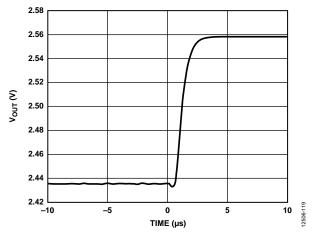
Figure 21. DAC Settling Time (100 Code Change, Rising Edge)
