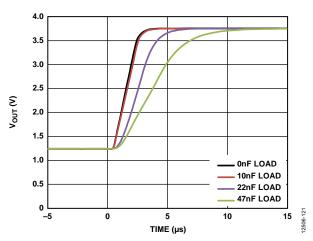
Figure 25. DAC Settling Time for Various Capacitive Loads
