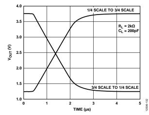
Figure 24. DAC Settling Time, Output Range =  $0 V to 2 \times V_{REF}$
