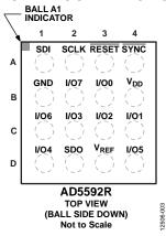
Figure 5. AD5592R 16-Ball WLCSP Pin Configuration
