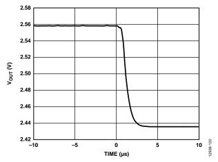
Figure 22. DAC Settling Time (100 Code Change, Falling Edge)
