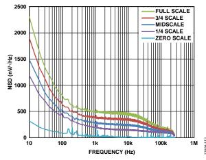
Figure 30. DAC Output Noise Spectral Density (NSD)
