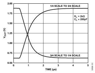
Figure 23. DAC Settling Time, Output Range =  $0 V \text{ to } V_{REF}$
