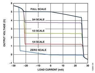
Figure 32. DAC Output Sink and Source Capability, Output Range =  $0 V to 2 \times V_{REF}$
