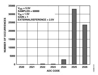
Figure 14. Histogram of ADC Codes,  $V_{DD} = 5.5 \text{ V}$
