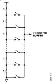
Figure 37. Simplified Resistor String Structure
