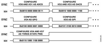
Figure 38. Typical Configuration Example
