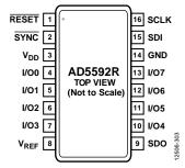
Figure 6. AD5592R 16-Lead TSSOP Pin Configuration
