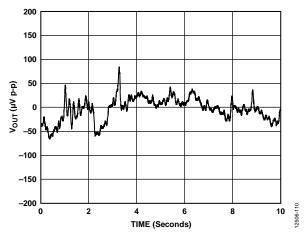
Figure 29. DAC 1/f Noise with Internal Reference
