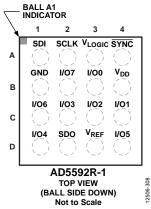
Figure 8. AD5592R-1 16-Ball WFCSP Pin Configuration
