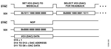
Figure 39. DAC Readback Operation
