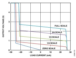
Figure 31. DAC Output Sink and Source Capability, Output Range =  $0 \text{ V to V}_{REF}$
