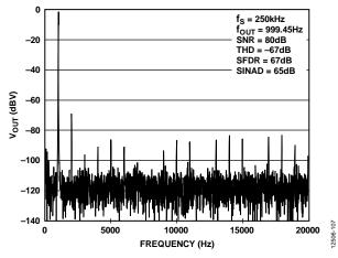
Figure 27. DAC Sine Wave Output, Output Range = 0 V to  $V_{REF}$ , Bandwidth = 0 Hz to 20 kHz
