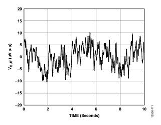
Figure 33. Internal Reference 1/f Noise
