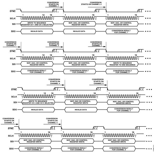
Figure 44. Changing a Multichannel, Repeating, ADC Conversion Sequence
