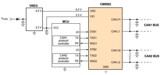
Figure 1. Simplified Application Diagram
