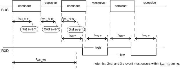
Figure 5. Wake-up Pattern Timing Illustration
