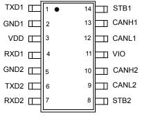
Figure 1. 14-Pin SOIC Pinout
