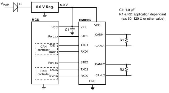
Figure 11. Single Supply Typical Application Schematic
