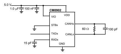
Figure 3. Timing Test Circuit
