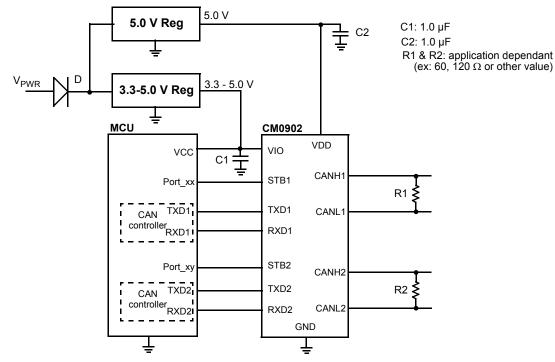
Figure 12. Dual Supply Typical Application Schematic
