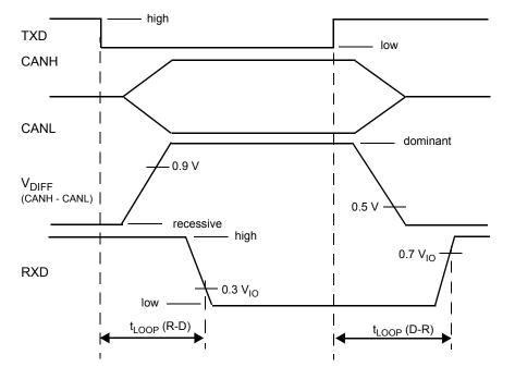
Figure 4. CAN Timing Diagram
