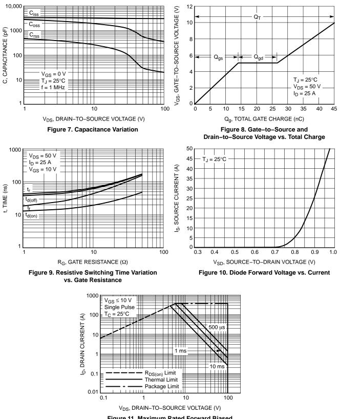
Figure 11. Maximum Rated Forward Biased Safe Operating Area
