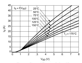
Figure 7. Forward Characteristics of Rev. Diode
