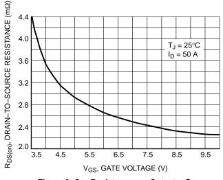
Figure 3. On-Resistance vs. Gate-to-Source Voltage
