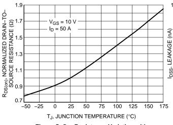
Figure 5. On–Resistance Variation with Temperature
