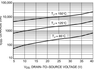
Figure 6. Drain-to-Source Leakage Current vs. Voltage
