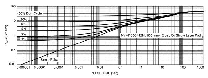
Figure 13. Thermal Characteristics
