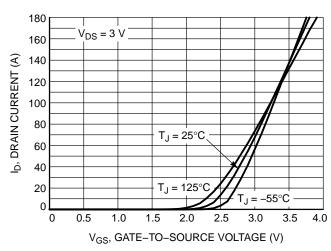
Figure 2. Transfer Characteristics
