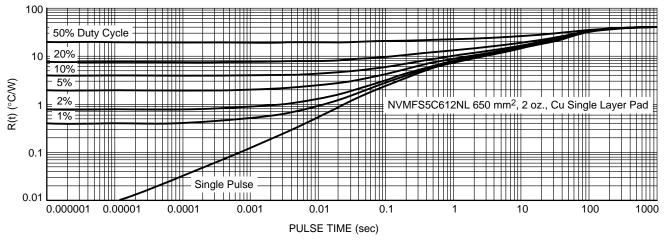
Figure 13. Thermal Characteristics
