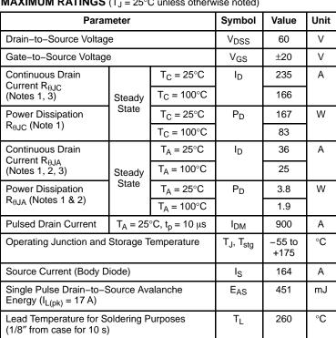
Stresses exceeding those listed in the Maximum Ratings table may damage the device. If any of these limits are exceeded, device functionality should not be assumed, damage may occur and reliability may be affected.
