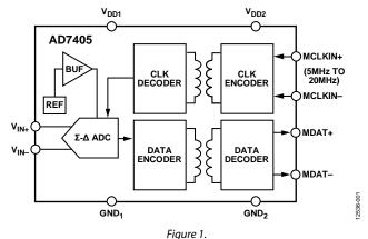
can be reconstructed with an appropriate digital filter to achieve 88 dB SNR at 78.1 kSPS. The LVDS input/output can use a 3 V to 5.5 V supply ( $V_{DD2}$ ).
