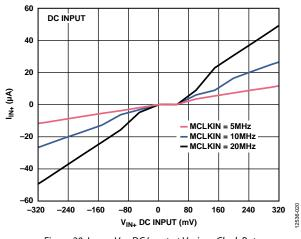
Figure 20. I<sub>IN+</sub> vs. V<sub>IN+</sub> DC Input at Various Clock Rates
