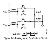
Because the AD7405 samples the differential voltage across its analog inputs, an input circuit provides low common-mode noise at each input attaining low noise performance.
