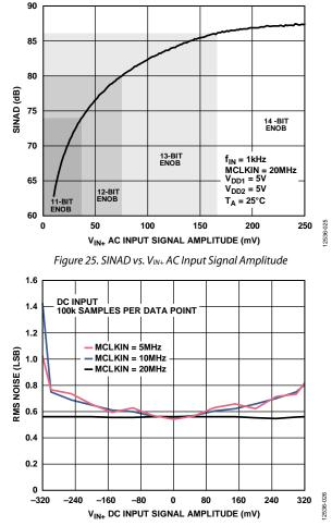
Figure 26. RMS Noise vs. V<sub>IN+</sub> DC Input Signal Amplitude
