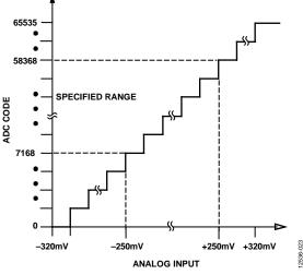
Figure 23. Filtered and Decimated 16-Bit Transfer Function
