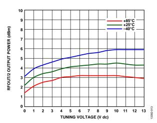
Figure 13. RFOUT/2 Output Power vs. Tuning Voltage
