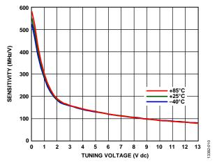
Figure 10. Sensitivity vs. Tuning Voltage
