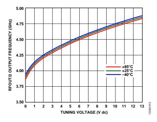
Figure 12. RFOUT/2 Output Frequency vs. Tuning Voltage
