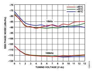
Figure 14. SSB Phase Noise vs. Tuning Voltage
