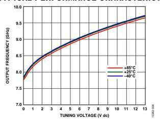
Figure 8. Output Frequency vs. Tuning Voltage
