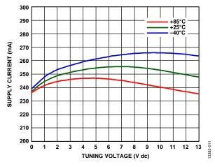
Figure 11. Supply Current (Icc) vs. Tuning Voltage
