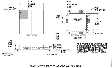
Figure 18. 32-Lead Lead Frame Chip Scale Package [LFCSP] 5 mm × 5 mm Body and 0.90 mm Package Height (HCP-32-1) Dimensions shown in millimeters
