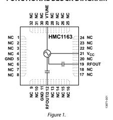
Because of the monolithic construction of the oscillator, the output power and phase noise performance are excellent over temperature.
