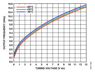
Figure 8. Output Frequency vs. Tuning Voltage
