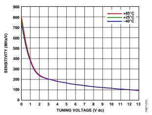
Figure 10. Sensitivity vs. Tuning Voltage
