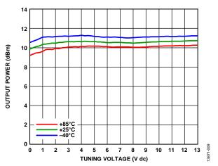
Figure 9. Output Power vs. Tuning Voltage
