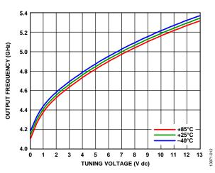
Figure 12. RFOUT/2 Output Frequency vs. Tuning Voltage
