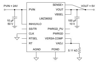
Figure 33. LMZ36002 Minimum External Component Application
