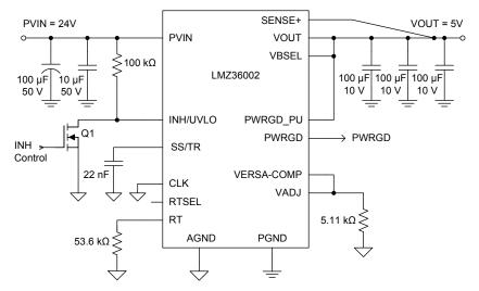
Figure 36. LMZ36002 Typical Schematic
