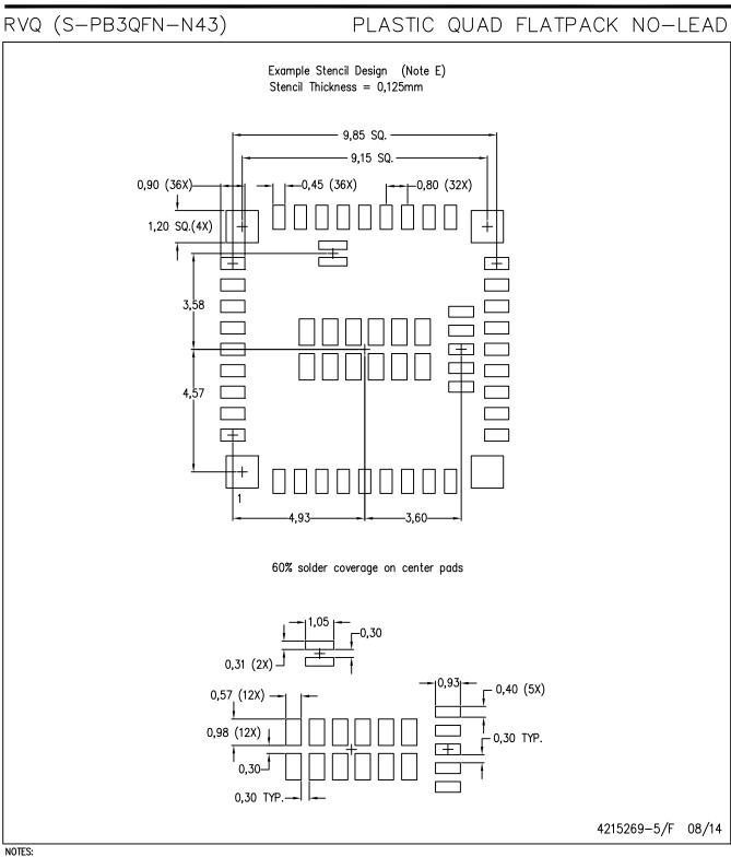
E. Laser cutting apertures with trapezoidal walls and also rounding corners will offer better paste release. Customers should contact their board assembly site for stencil design recommendations. Refer to IPC 7525 for stencil design considerations.
