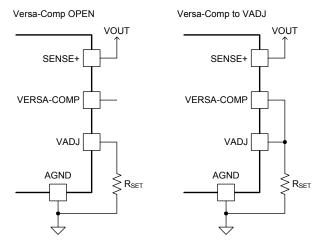
Figure 25. Versa-Comp Configurations
