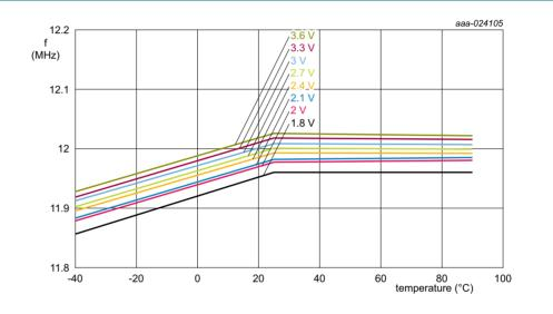
Conditions: Frequency values are typical values. 12 MHz  $\pm$  1.5 % accuracy is guaranteed for 2.7 V  $\leq$  V<sub>DD</sub>  $\leq$  3.6 V. Variations between parts may cause the IRC to fall outside the 12 MHz  $\pm$  1.5 % accuracy specification for voltages below 2.7 V.
