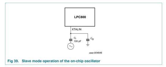
In slave mode the input clock signal should be coupled with a capacitor of 100 pF (Figure 39), with an amplitude between 200 mV (RMS) and 1000 mV (RMS). This corresponds to a square wave signal with a signal swing of between 280 mV and 1.4 V. The XTALOUT pin in this configuration can be left unconnected.
