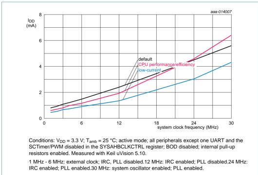
Fig 23. Active mode: CoreMark power consumption IDD
