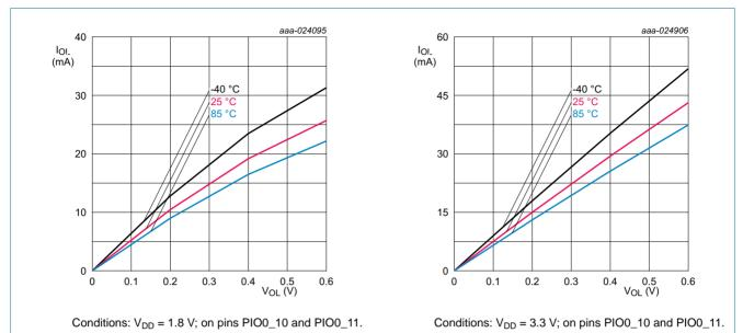
Fig 25. I<sup>2</sup>C-bus pins (high current sink): Typical LOW-level output current I<sub>OL</sub> versus LOW-level output voltage V<sub>OL</sub>
