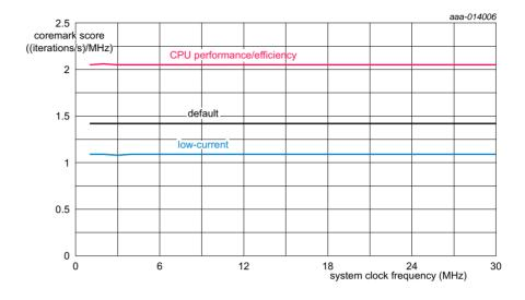
Conditions: V<sub>DD</sub> = 3.3 V; T<sub>amb</sub> = 25 °C; active mode; all peripherals except one UART and the SCTimer/PWM disabled in the SYSAHBCLKCTRL register; BOD disabled; internal pull-up resistors enabled. Measured with Keil uVision 5.10.
