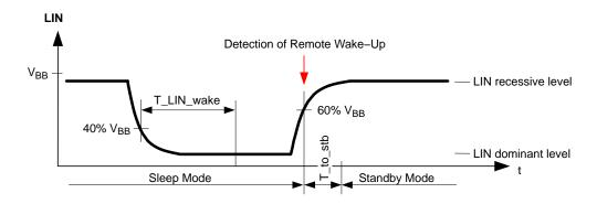
Figure 5. Remote (LIN) Wake-up Detection
