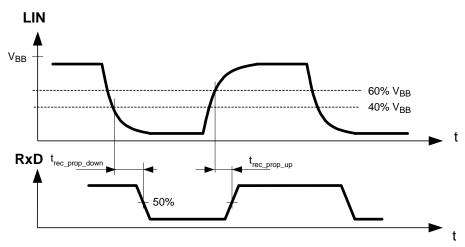
Figure 9. LIN Receiver Timing
