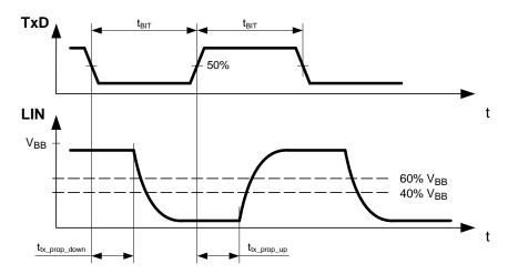
**Figure 7. LIN Transmitter Timing**
