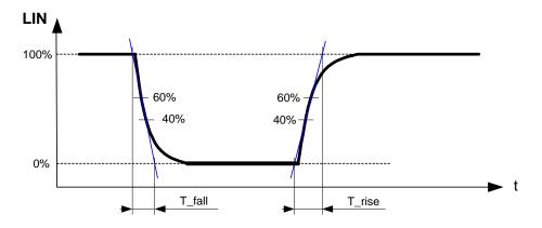
Figure 8. LIN Transmitter Rising and Falling Times
