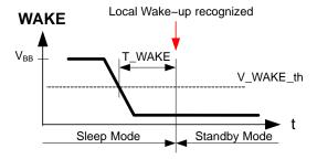
Figure 4. Local Wake-up Detection
