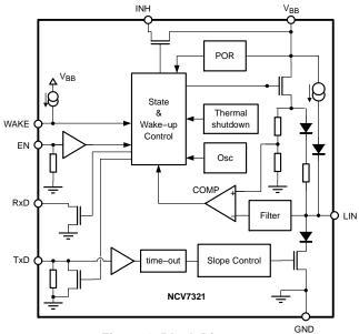
Figure 1. Block Diagram
