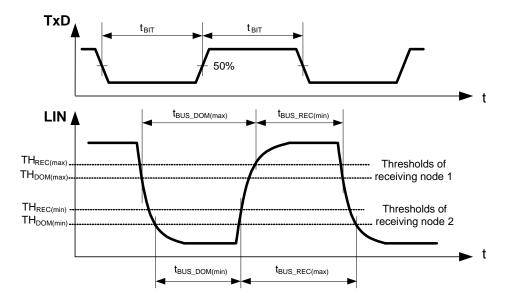
Figure 6. LIN Transmitter Duty Cycle
