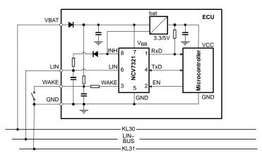
Figure 2. Typical Application Diagram for a Master Node
