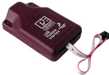
Figure 10-1: P&E's USB Multilink (USB-ML-12 shown)
