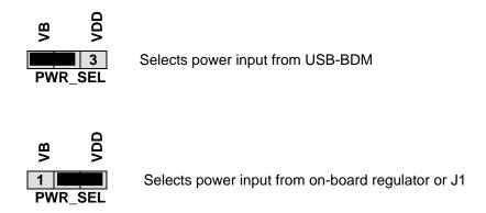
**NOTE:** Set PWR\_SEL jumper to VB during application development. Use barrel connector input (PWR) to support LIN functionality if needed.
