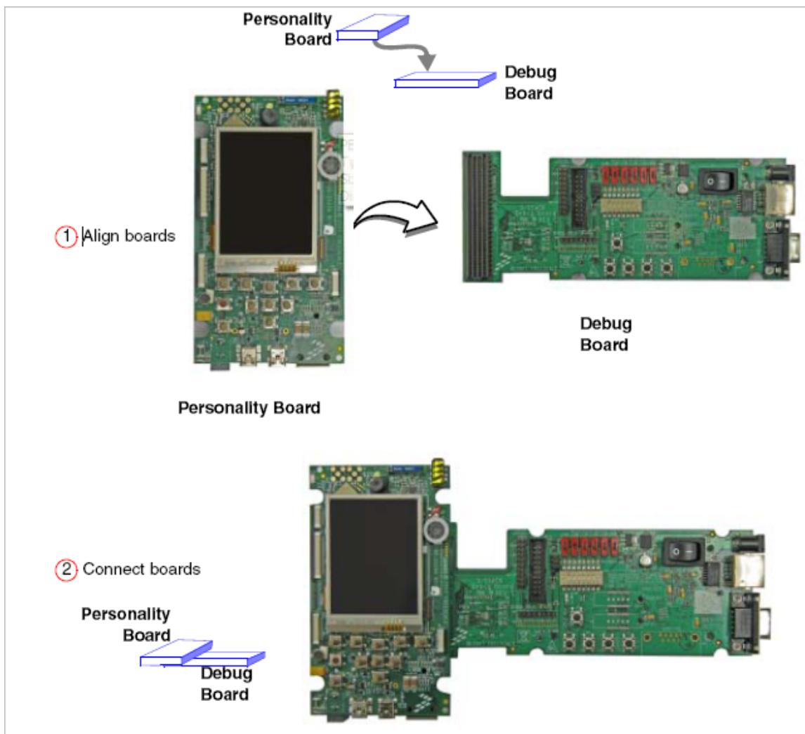
Figure 3-2 Install Personality Board onto Debug Board
