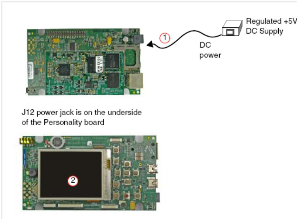
**Figure 3-6 Connect Personality Board to Power Supply**
