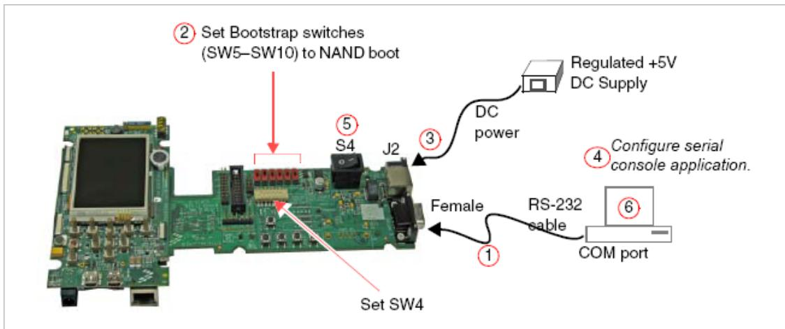
**Figure 3-4 Connecting the Platform to Your PC**
