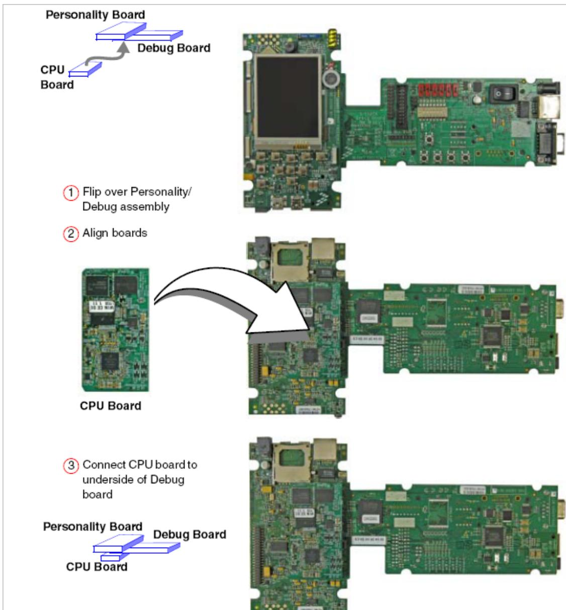
Figure 3-3 Align CPU Board and Debug/Personality Board
