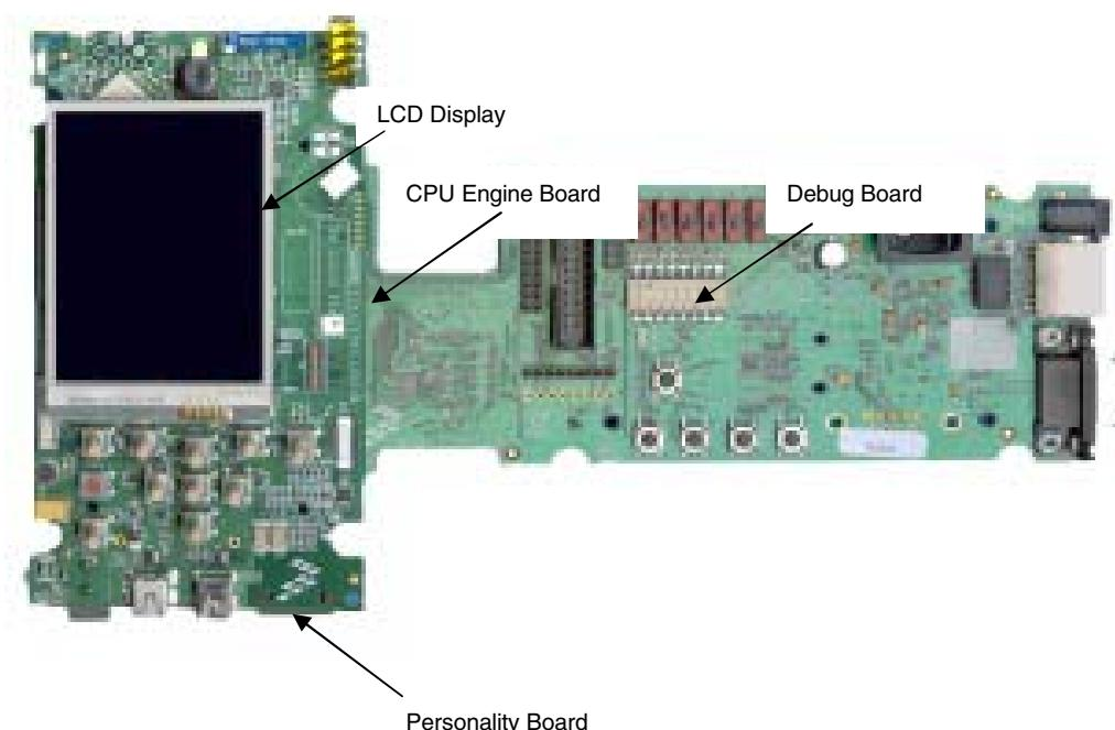
**Figure 1-1 Major Components of the 3-Stack System**
